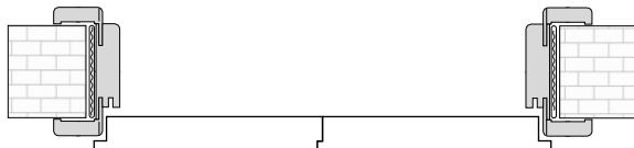
MODULOVÉ A PLOCHÉ DVERE S REGULOVANOU ALEBO BLOKOVOU ZÁRUBŇOU DVERE SA SKLADAJÚ Z FALCOVÉJ ČASŤI A PROTIFALCA
